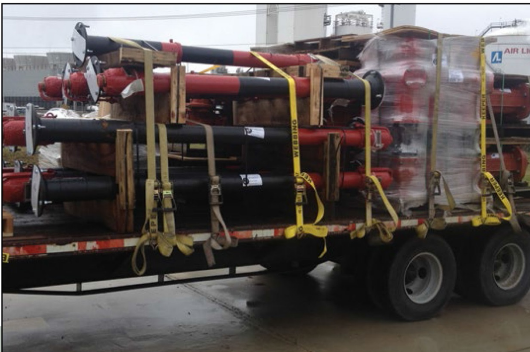
POST INDICATOR VALVE & POST
