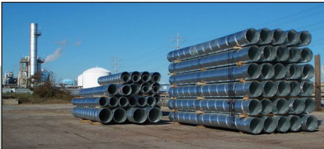
GALVANIZED CORRUGATED METAL PIPE
